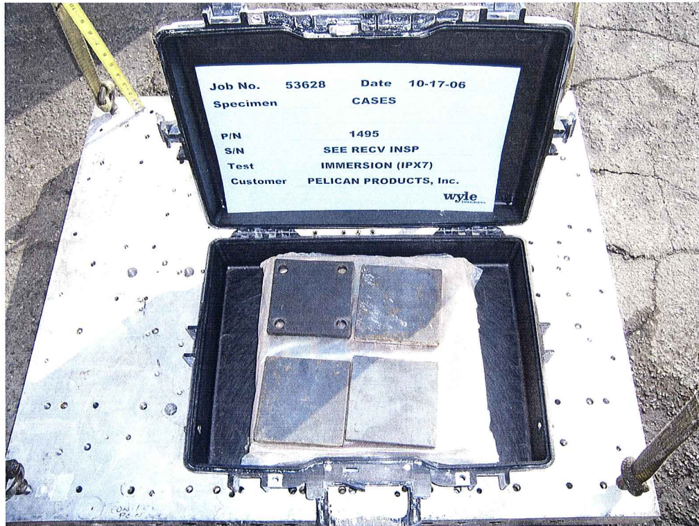
Photograph 3 Immersion Test Setup
