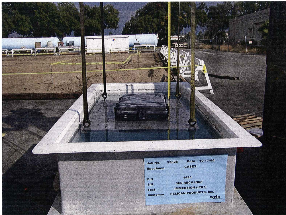
Photograph 4 Immersion Test Setup
