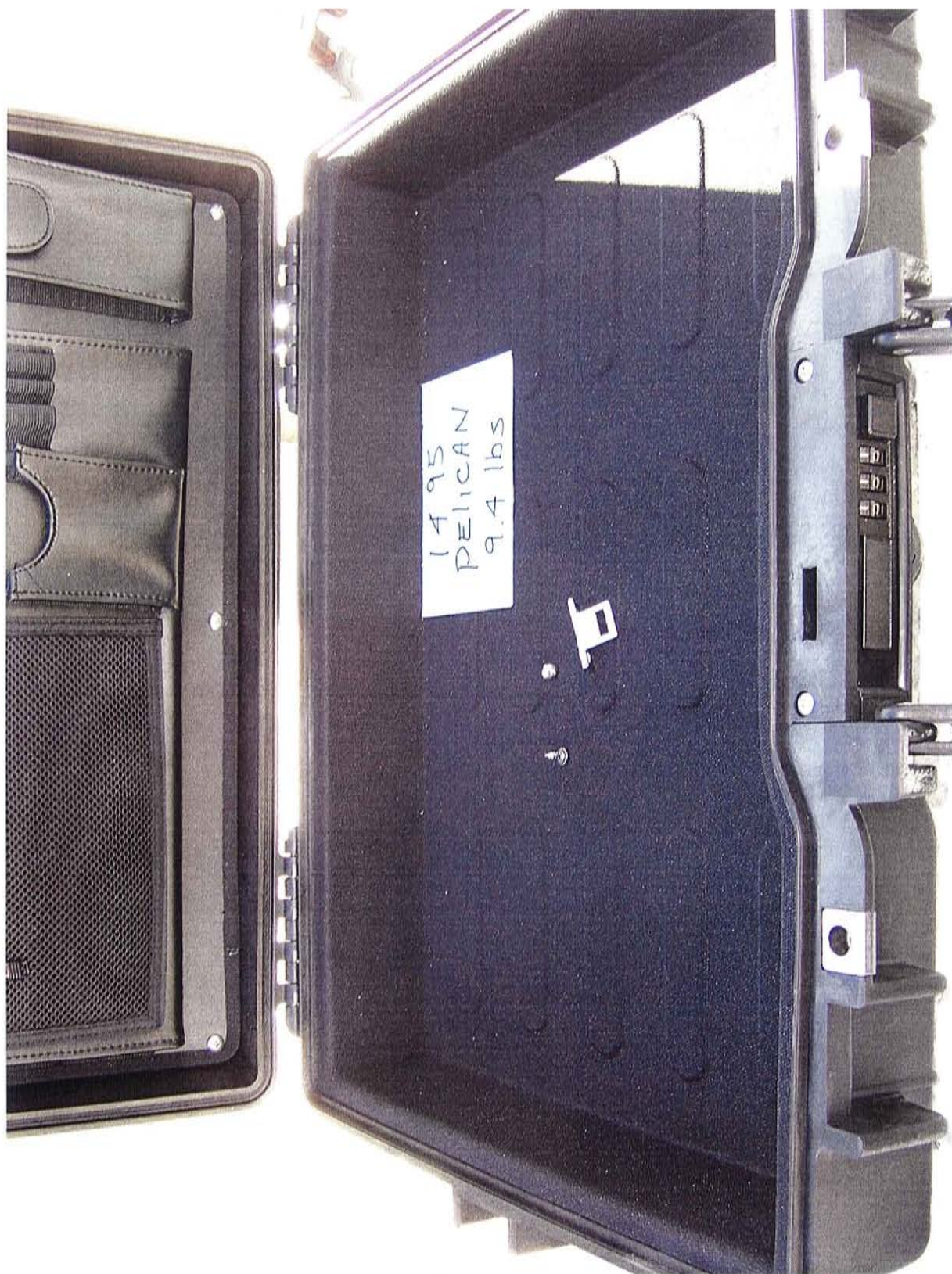
Photograph 11 Post Near End Impact – Stripped Locking Latch
