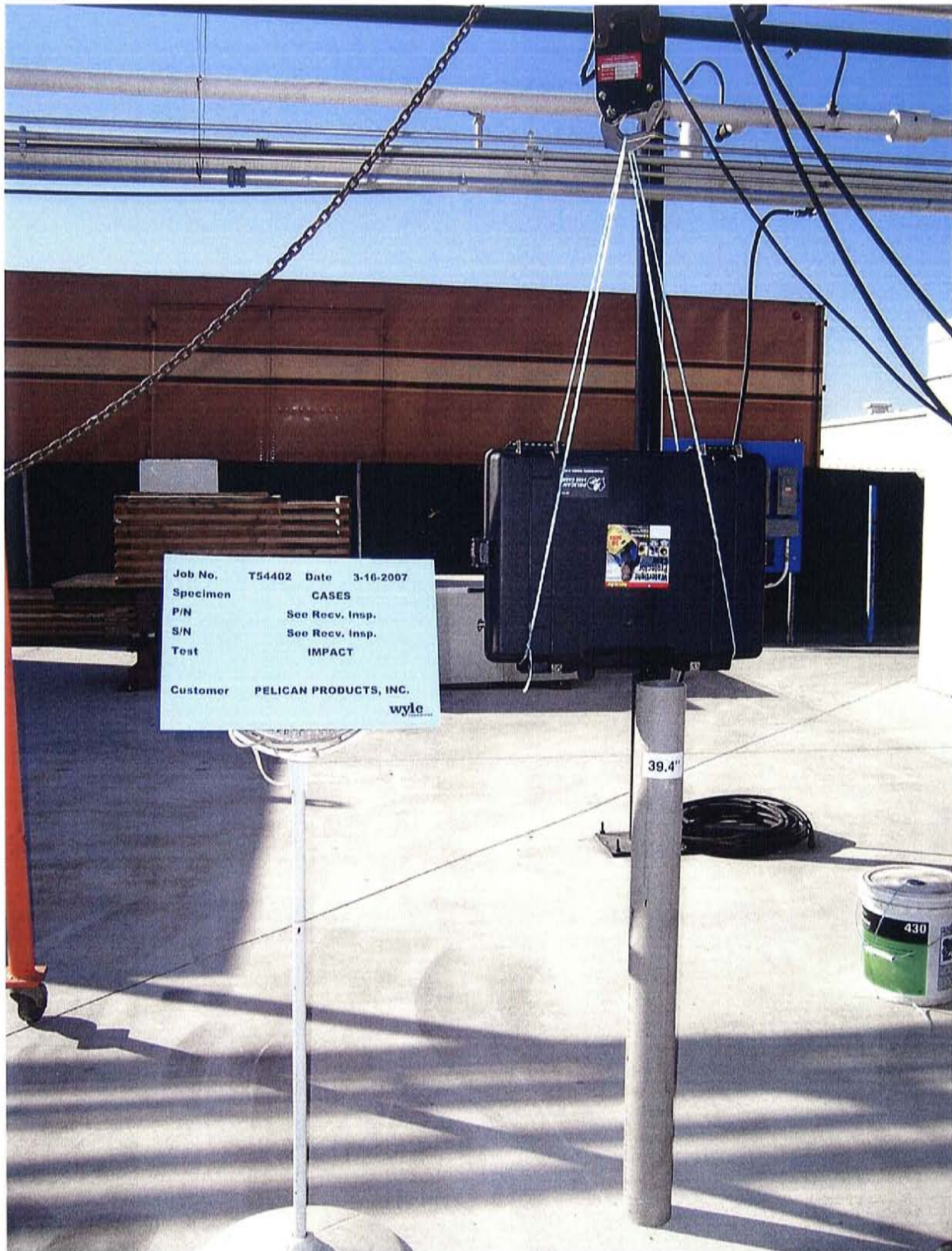
Photograph 9 Impact Test Setup (Near End Impact)
