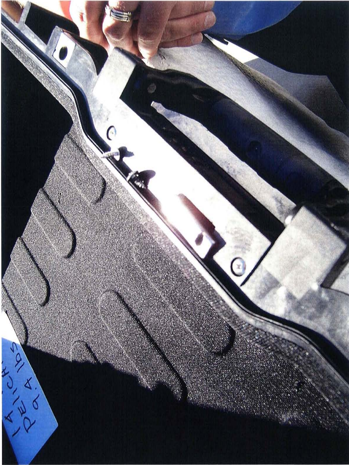
Photograph 10 Post Near End Impact – Stripped Locking Latch
